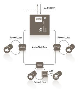
Note: All PowerLoop cables must be shielded.
