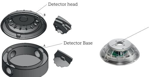
**NOTE!** There is a mark in the plastic that indicates the detector's 30° field of view. This must point in the direction from the wall towards the inside of the bracket.
