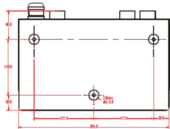
Leave 80 mm clearance at top and bottom of docking station for access
